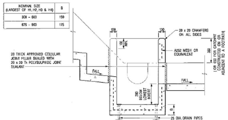
**Details of Catchpit with Sand Trap**
